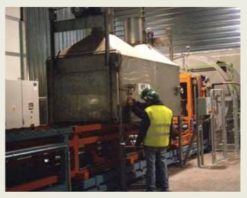
*Muffle furnace in BCD remediation plant in Spolana Neratovice.*
