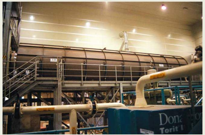
Indirect thermal desorption unit in Spolana Neratovice served for evaporization of persistent pollutants from contaminated debries and soil into processing oil.
