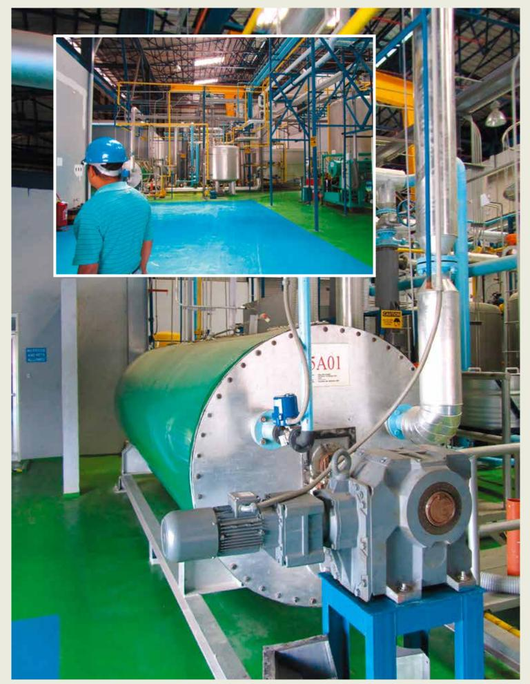
Sodium Reduction (SR) facility used for destruction of PCB oils in Philippines.
