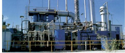
Liquid and solid wastes are placed into the TRBP, which is then heated to approximately 600°C in a hydrogen-rich (oxygen deficient) atmosphere. Contaminants that volatilize from the solids and liquids are then swept into the GPCR reactor for destruction.
