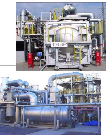
Mobile Liquid Waste Pre-heater for GPCR Plant
